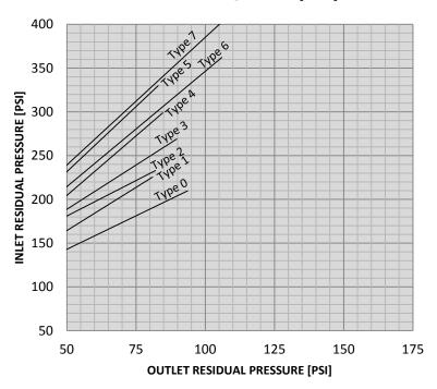
2.5" IE2600 Inline Body Inlet vs. Outlet Pressure @ Static Flow
