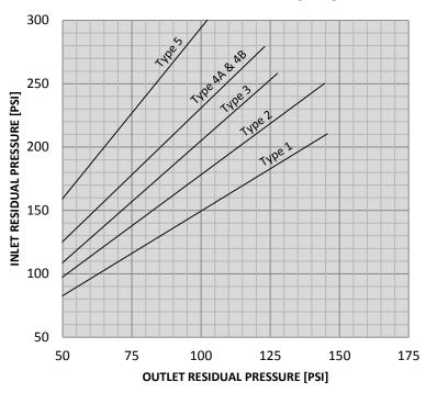
1.5" 90-FS-PRV Angle Body Inlet vs. Outlet Pressure @ 200-250 [GPM]
