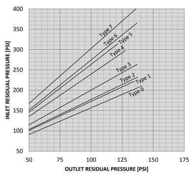
2.5" 90-FS-PRV Inline Body Inlet vs. Outlet Pressure @ 300-400 [GPM]
