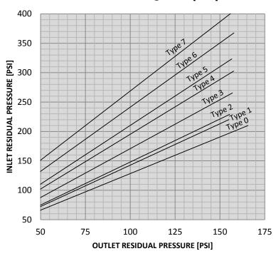
2.5" 90-FS-PRV Angle Body Inlet vs. Outlet Pressure @ 200-300 [GPM]
