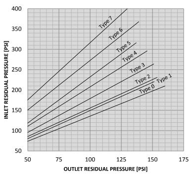
2.5" 90-FS-PRV Angle Body Inlet vs. Outlet Pressure @ 400-500 [GPM]
