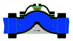
To open the valve, the water or air trapped within the upper chamber is released into atmosphere or into the downstream of the valve, into the pipeline.
