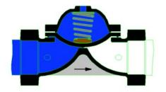
To close the valve, water or air pressure is induced into the upper chamber forcing the diaphragm to close against the weir within the valve and thereby stopping the flow of the liquid or gas within the pipeline.
