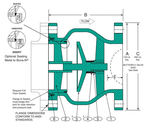
Note: Plug 3 & spring 4 compressed are shown in Open Position.
