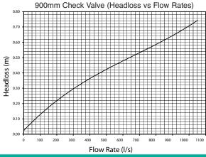
Sample Flow Rate vs Headloss Graphs. Other size charts available upon request. Based on flow testing at Utah State University.
