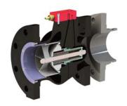
This 4 inch In-line Valve is rated for 1,200 gpm maximum. As an added environmental protection, the 354GF In-line Pressure Control Valve features a manual bleed valve on the Pilot Block to which a bleed hose can be easily attached so that bleeding air from the Valve does not result in a fuel spillage.
