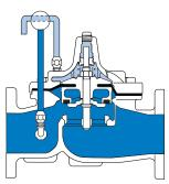
**Full Open Operation** When pressure in the diaphragm chamber is relieved to zone of lower pressure under the valve. Flow in either direction is permitted.
