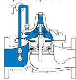
**Tight Closing Operation** When pressure from the valve inlet (or an equivalent independent operating pressure) is applied to the diaphragm chamber, the valve closes drip-tight.
