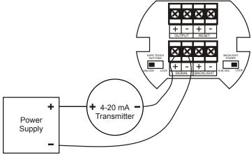
Figure 2. Input Connections without Backlight
