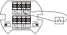
Figure 5. Reset Connections
