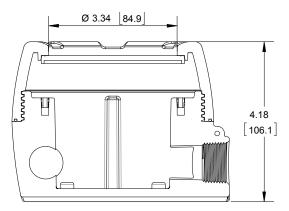
Figure 11. Enclosure Dimensions – Side Cross Section View
