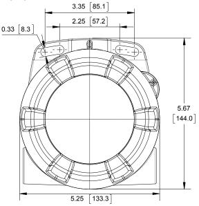
Figure 10. Enclosure Dimensions – Front View
