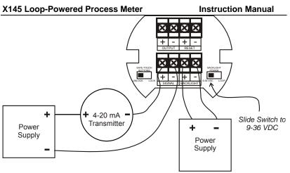
Figure 4. Input Connections with Externally-Powered Backlight
