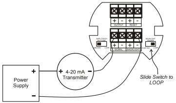
Figure 3. Input Connections with Loop-Powered Backlight
