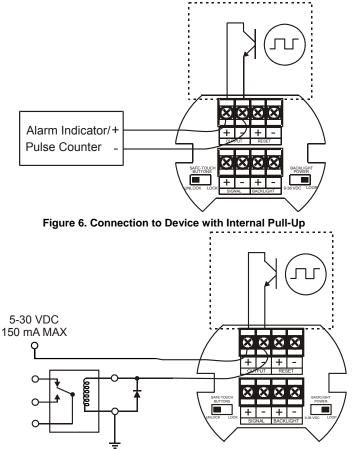
Figure 7. Output Connections
