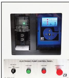
The Cla-Val PC-22D provides control of the pump and pump control valve, preventing surges in the system when the pump starts or stops. It consists of a pre-wired electrical control panel employing a programmable valve controller to sequence the pump and pump control valve during all modes of operation. Provides added protection to the pumping system from damage caused by mechanical, hydraulic or power failure.
